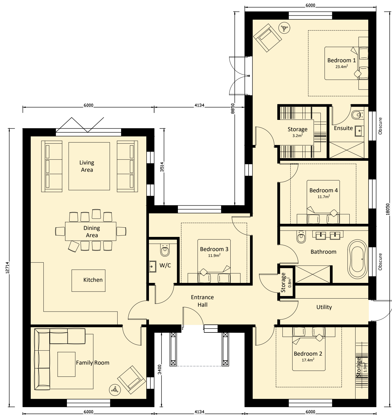
PLOTS 2 AND 3 GROUND FLOOR PLAN 180.2m 2 (1,940sq.ft) 1 Storey, 4Bedroom, 8Persons
